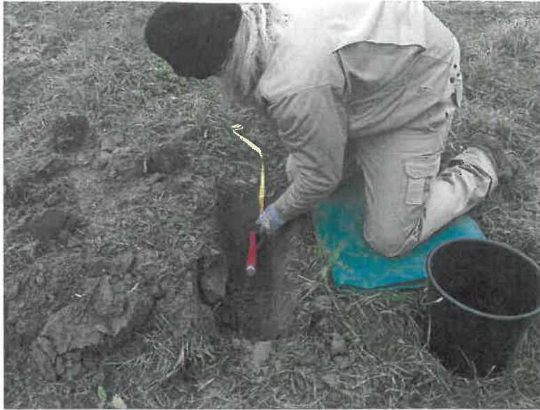
Fig. 3.2. Volumetric sampling. The slide hammer is used to insert the core, dug out to prevent shearing of pieces, and split apart for placement of samples in soil cans.
