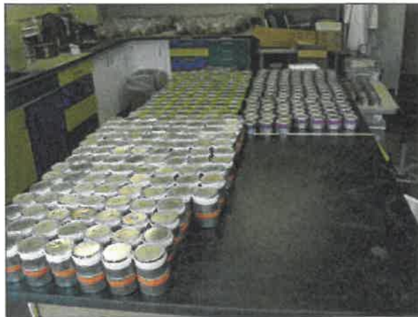
Fig. 3.3. The soil cans are filled and taped for later weighing in the laboratory.
