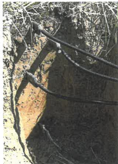
Fig. 3.6. Network of TDT sensors at different depths.
